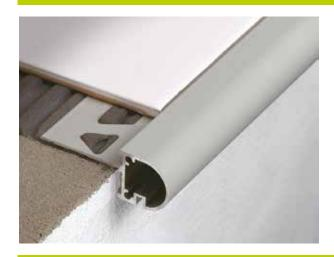
Perimeter profile that finishes and protects the exposed concrete edge of balconies and terraces incorporating a symetrically shaped upper edging trim designed to frame the tiles surface. Particularly suitable for tiling on pre-existing floors. Includes an intergrsted "drip-lip". It is important to leave a space between elements for thermal expansion and covered by the covering cap.
